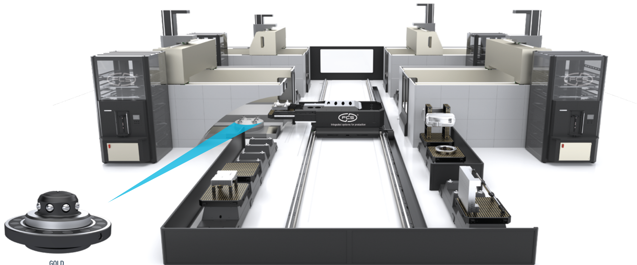
Flexible manufacturing system (FMS): machine tools feeding by a pallet changer system
